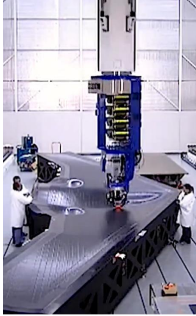
Figure 3. Automated Fiber Placement application [6]
